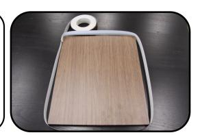
Apply the edge banding on the contour of the door starting where the edge is less visible. Do not start on a corner. The extra edge banding to be cut should be on the interior of the door.
