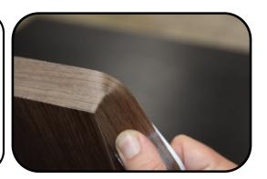
Using the precision knife, remove the excess of edge banding on the back of the door.
