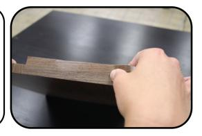
When applying the edge banding, it is important that it does not exceed on the front panel. Leave a space of 1 mm as shown in the photo, this will prevent it from catching and peeling.
