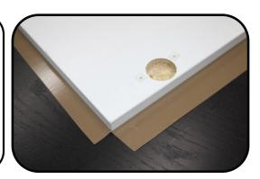
the Wrap MK around the edges. Using the felt squeegee at a 45 degree angle on the edge will help the Wrap MK to mold properly.
